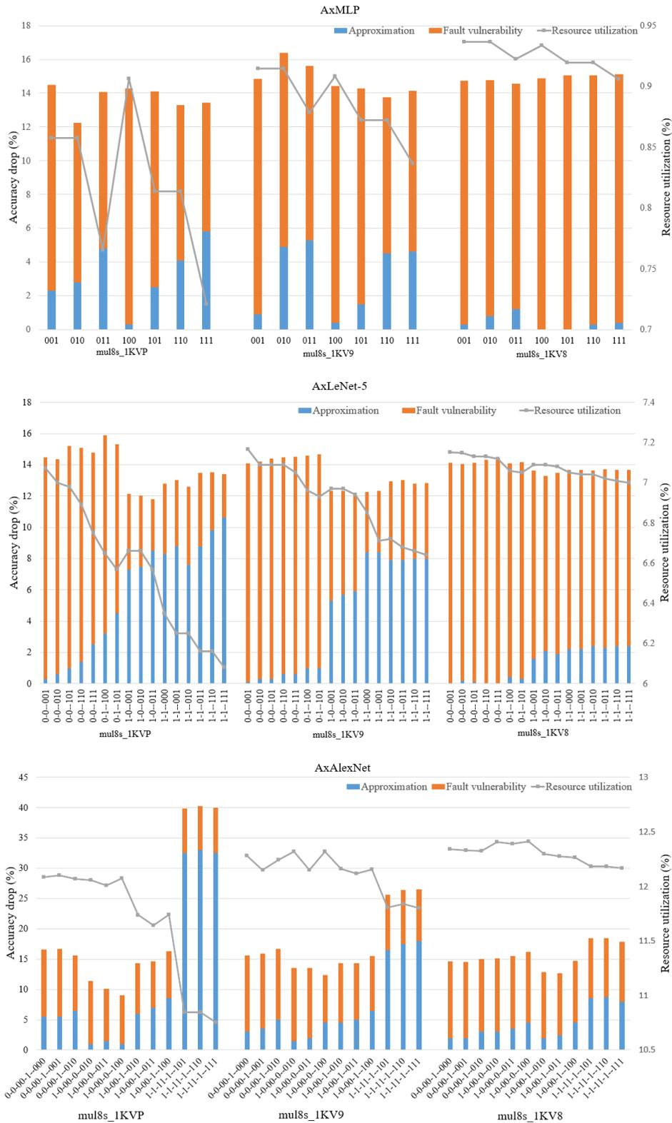
Fig. 4: Reports of accuracy drop (due to approximation for different configurations), fault vulnerability, and resource utilization of (a) 3-layer MLP network, (b) LeNet-5 and (c) AlexNet
