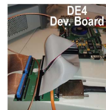
Figure 3.4.S1: The frequency-reference measurement setup (top) consists of a motherboard carrying 4 samples. This is placed in an oven, and the samples are controlled by an FPGA. The PC (via a DAQ card) is only used to control the measurement setup.
