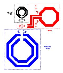
Figure 4.4: Layout placement for inductors and transistors
