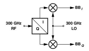
Figure 6.3: Homodyne receiver with IQ seperated input
