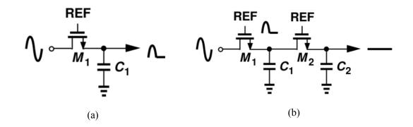
Figure 3.29: Single stage sampling for phase detector (a), master slave sampling for phase detector (a(b)
