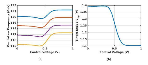
Figure 3.15: 120 GHz VCO oscillation frequency with respect to control voltage and capacitor banks (a), single ended peak-to-peak swing (b)
