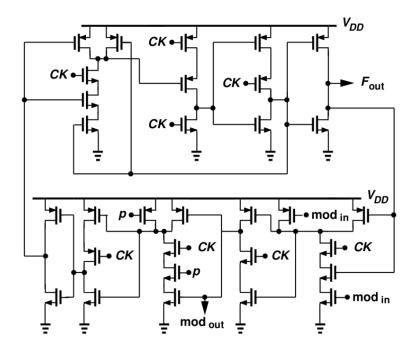
Figure 3.27: 2/3 divider cell circuit diagram implemented with TSPC logic
