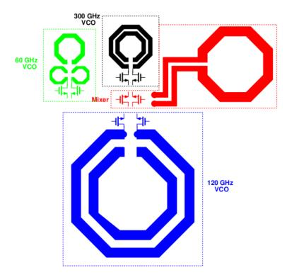
Figure 4.7: Layout placement for 60 GHz VCO inductors in the whole floorplan
