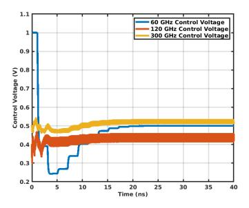
Figure 5.1: Control Voltages for different PLL's when locking
