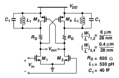
Figure 6.14: IF amplifier with shunt peaking and PMOS cross-coupled pair
