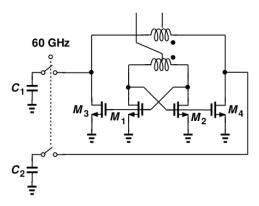
Figure 3.14: Modulation of 120-GHz VCO with 60-GHz VCO
