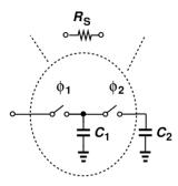
Figure 3.31: Equivalent circuit for an MSSPD
