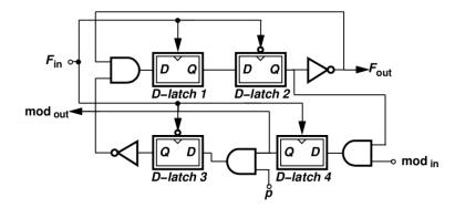
Figure 3.26: 2/3 divider cell logic diagram
