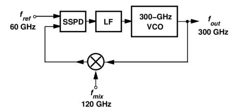
Figure 2.4: 300-GHz PLL employing a mixer to reduce frequency input to SSPD and uses a 60-GHz reference
