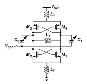
Figure 3.17: 60 GHz VCO schematic
