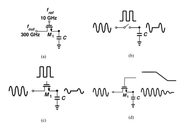
Figure 2.3: Subsampling phase detector with an NMOS and a capacitor (a) an ideal sampler with square wave reference waveform (b), sampling transistor with square-wave reference (c), sampling with finite rise-fall time signal (d)
