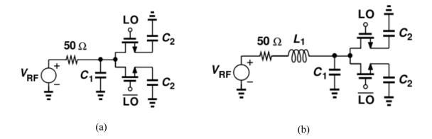
Figure 6.9: Mixer directly connected to 50  $\Omega$  input (a), mixer connected to input with a resonating inductor (b)
