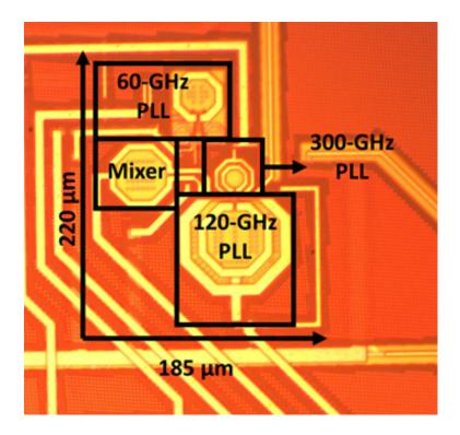
Figure 5.12: 300 GHz PLL chip micrograph. The active area is 180 µm x 220 µm
