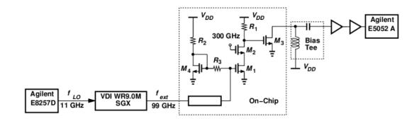
Figure 5.18: 300 GHz PLL output measurement setup for phase noise analysis
