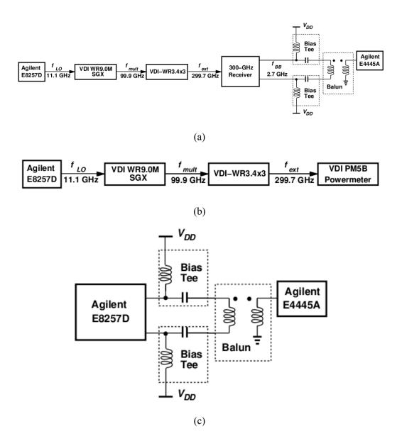
Figure 6.24: Measurement setups for gain measurement (a) and input power measurement (b) and loss calibration (c)
