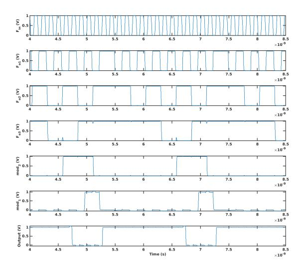
Figure 3.28: Simulation result for the divide-by-15 circuit with all 2/3 divider cell and mod outputs
