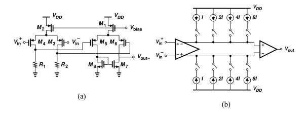
Figure 3.9: Gain stage design (a), programmable currents added to control output DC level (b)
