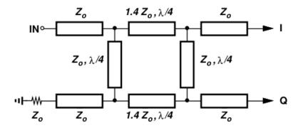
Figure 6.2: Quadrature coupler with quarter wavelength transmission lines
