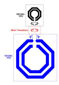
Figure 4.3: Layout placement for VCO inductors and transistors
