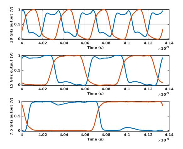
Figure 3.23: 60-GHz divide-by-8 outputs at each step
