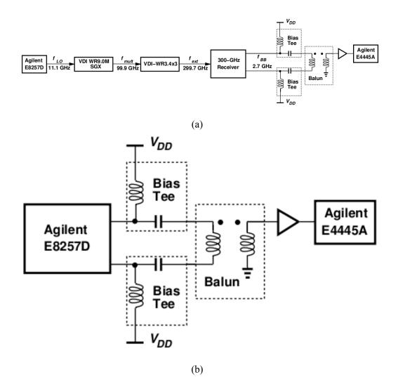
Figure 6.25: Measurement setups for noise figure measurement, gain measurement (a) and loss calibration (b)
