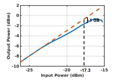
Figure 6.27: P<sub>1dB</sub> measurement at 1 GHz
