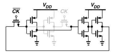
Figure 3.22: 60-GHz divider with a strong feedforward path
