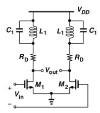
Figure 6.13: IF amplifier with shunt peaking
