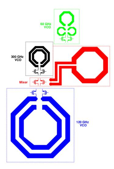
Figure 4.8: Final layout placement for 60 GHz VCO inductors in the whole floorplan
