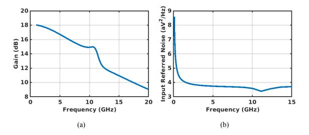
Figure 6.21: Baseband amplifier gain(a) and input referred noise (b)
