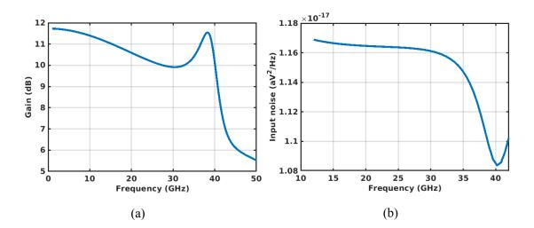
Figure 6.15: IF amplifier gain(a) and input referred noise (b)
