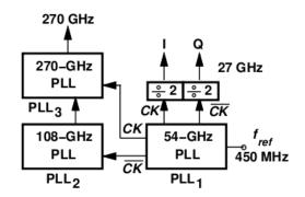
Figure 6.5: Clock generator for the heterodyne receiver
