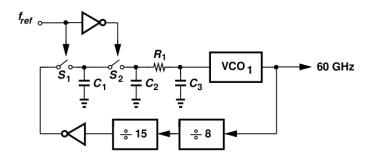
Figure 3.16: 60GHz PLL schematic
