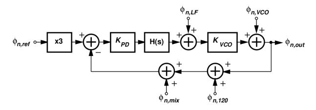
Figure 3.10: Small signal model for phase noise analysis
