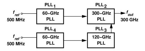
Figure 3.11: A system proposition for uncorrelating phase noise
