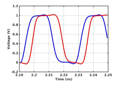
Figure 6.17: Transient waveforms for quadrature divider
