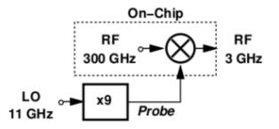
Figure 5.8: On-Chip harmonic mixer and external frequency multiplier for the test setup
