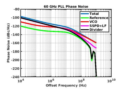
Figure 5.2: 60-GHz PLL's output phase noise and its noise contributors
