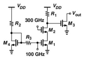
Figure 5.10: Harmonic mixer and output buffer and the current mirror
