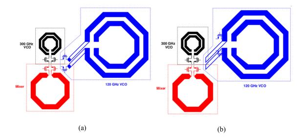
Figure 4.2: 120 GHz VCO inductor on the right side of 300 GHz VCO inductor and mixer inductor. 120 GHz VCO transistors are close to the other transistors (a), 120 GHz VCO transistors are at the VCO inductor (b)
