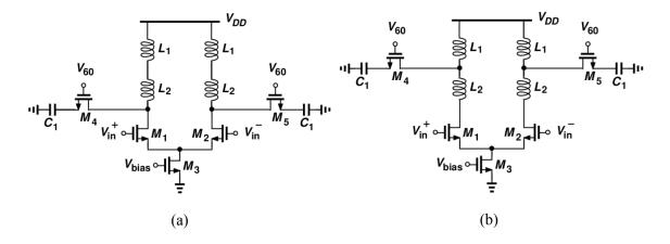
Figure 4.5: Different placements for the sub-sampler, right at the transistors (a), after travelling through some path (b)
