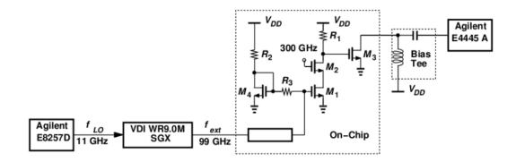
Figure 5.16: 300 GHz PLL output measurement setup for spectrum analysis
