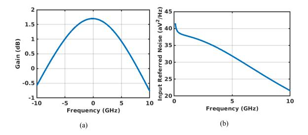
Figure 6.19: IF mixer gain(a) and output noise (b)
