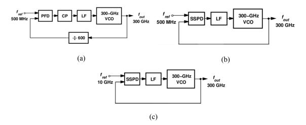
Figure 2.2: A standard PLL design with 300 GHz VCO, a phase detector, charge pump, loop filter and a divide-by-600 circuit (a), Subsampling PLL with 500 MHz reference (b), Subsampling PLL with 10 GHz reference (c)
