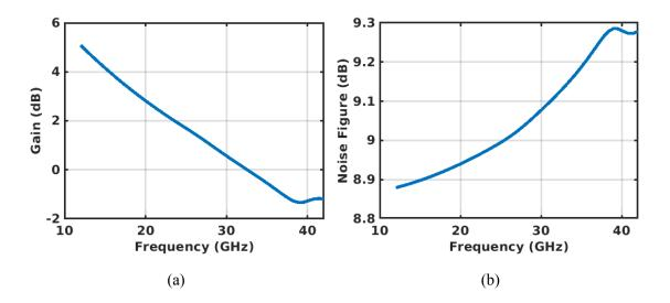
Figure 6.11: RF mixer gain(a) and noise figure for downconverted signal (b)
