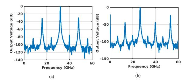
Figure 3.24: Maximum divider frequency at SS corner (a), minimum divider frequency at FF corner (a(b)
