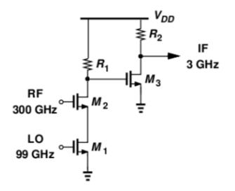
Figure 5.9: Harmonic mixer and output buffer
