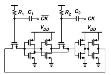
Figure 3.21: Modified divide-by-2 circuit for 60 GHz input
