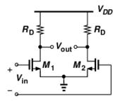
Figure 6.12: Basic differential as IF amplifier
