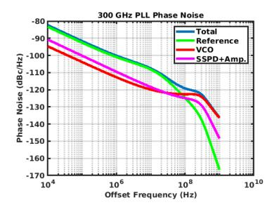
Figure 5.4: 300-GHz PLL's output phase noise and its noise contributors
