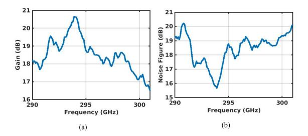
Figure 6.26: Gain (a) and noise figure (b) measurement results
