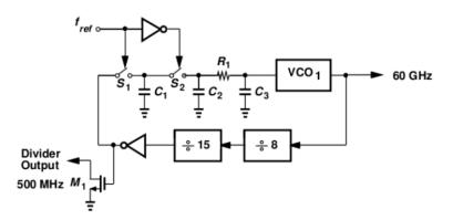
Figure 5.13: 500-MHz divider output measurement setup
