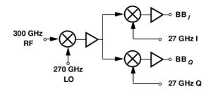
Figure 6.4: Heterodyne quadrature receiver
