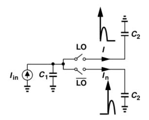
Figure 6.7: Mixer current waveforms going into the load capacitors
