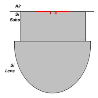
Figure 5.7: On-chip antenna with silicon lens to enhance gain
