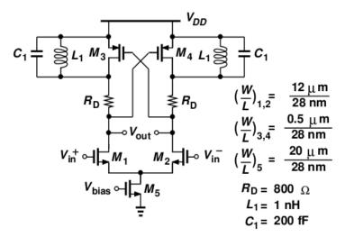
Figure 6.20: Baseband amplifier schematic
