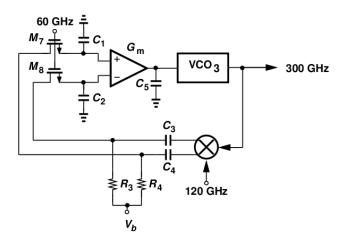
Figure 3.2: Proposed 300-GHz PLL architecture
