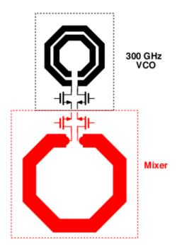
Figure 4.1: An idealized placement for VCO inductor and mixer inductor in 300 GHz PLL loop
