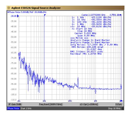
Figure 5.19: 300 GHz PLL downconverted phase noise.  $f_{ext}$ = 99.288 GHz
