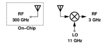
Figure 5.6: Measurement setup with an on-chip antenna
