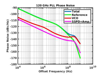
Figure 5.3: 120-GHz PLL's output phase noise and its noise contributors
