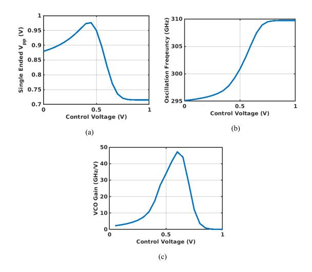
Figure 3.7: Single ended peak to peak swing with respect to control voltage (a), VCO frequency with respect to control voltage (b), VCO gain with respect to control voltage (c)
