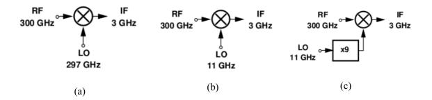
Figure 5.5: Fundamental mixer with 297-GHz LO input to generate 3 GHz IF output (a), harmonic mixer which uses 27th harmonic with 11-GHz LO input to generate 3 GHz IF output (b), harmonic mixer which uses 3rd harmonic and x9 frequency multiplier to move input frequency from 11 GHz to 99 GHz to generate 3 GHz IF (c)
