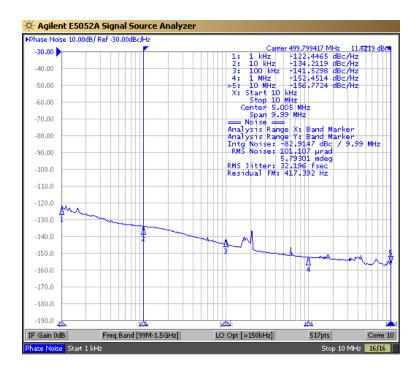
Figure 5.15: 500 MHz locked signal phase noise
