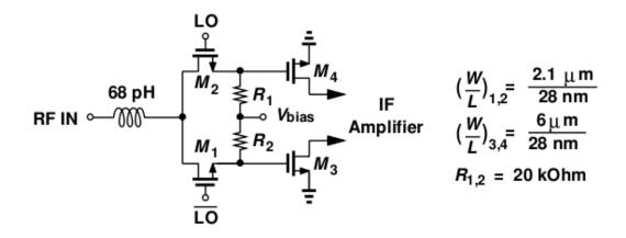
Figure 6.10: RF mixer schematic with component values
