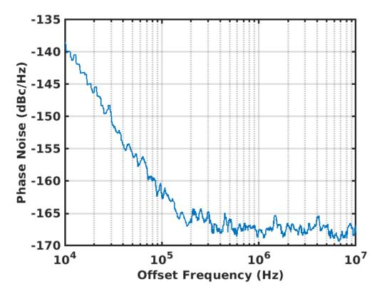
Figure 5.20: Phase noise of the crystal oscillator
