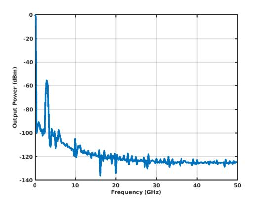
Figure 5.11: Downconverted output at 3 GHz with -55 dBm output power
