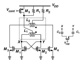
Figure 3.13: 120-GHz VCO schematic
