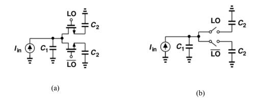
Figure 6.6: RF mixer simplified (a), approximate structure to model gain (b)
