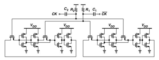
Figure 6.16: Complete divider schematic for quadrature separation
