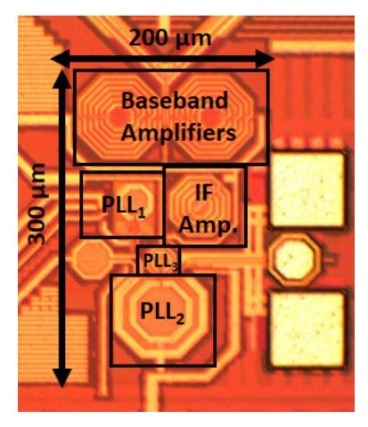
Figure 6.22: Chip photo for 300-GHz receiver
