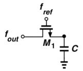
Figure 3.5: Subsampling stage in 300-GHz PLL
