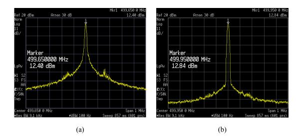
Figure 5.14: Spectrum of unlocked (a) and locked (b) 500-MHz divider outputs (b)
