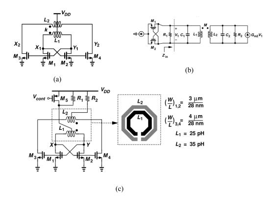
Figure 3.6: Buffer feedback oscillator (a), simplified small-signal analysis (b), BFO converted into a VCO with the help of  $M_5$  and physical implementation of transformer (c)
