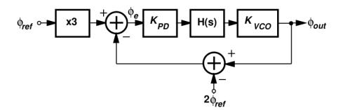
Figure 3.3: Small signal phase equivalent of 300-GHz PLL
