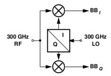
Figure 6.1: Homodyne receiver with IQ seperated clocks
