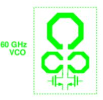
Figure 4.6: Layout placement for VCO inductors in 60 GHz VCO
