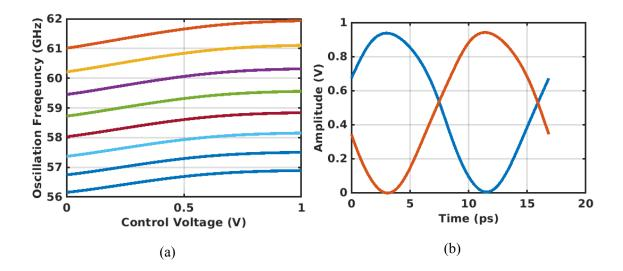
Figure 3.18: 60 GHz VCO oscillation frequency with respect to control voltage and capacitor banks (a), output swings in time domain (b)
