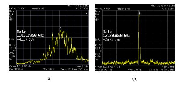
Figure 5.17: Spectrum of unlocked (a) and locked (b) 300-GHz PLL outputs (b) For both cases  $f_{ext}$ = 99.54 GHz
