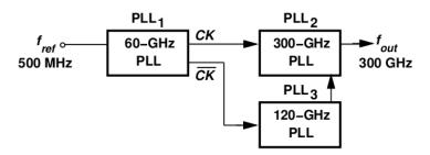
Figure 3.1: Proposed system architecture including a PLL at 60 GHz, 120 GHz and 300 GHz
