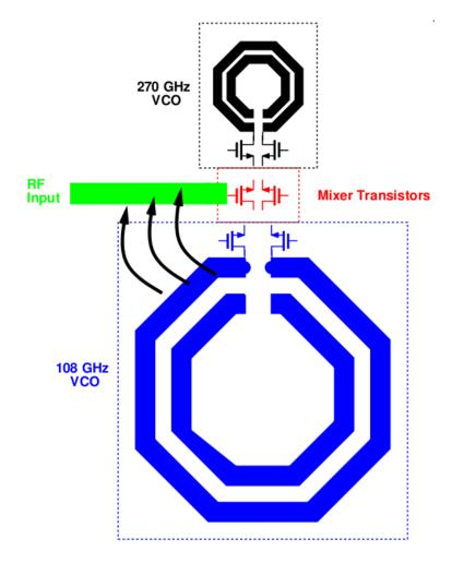
Figure 6.23: Coupling path for 108-VCO
