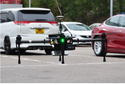
Fig. 5: Experimental set-up for acquiring stereo road images.
