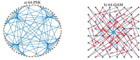
Fig. 5. Optimized sequence for 64-PSK and 64-QAM.
