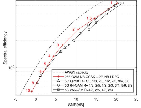
Fig. 9. Spectral efficiency of NB-CCSK(256) with 256-APSK modulation
