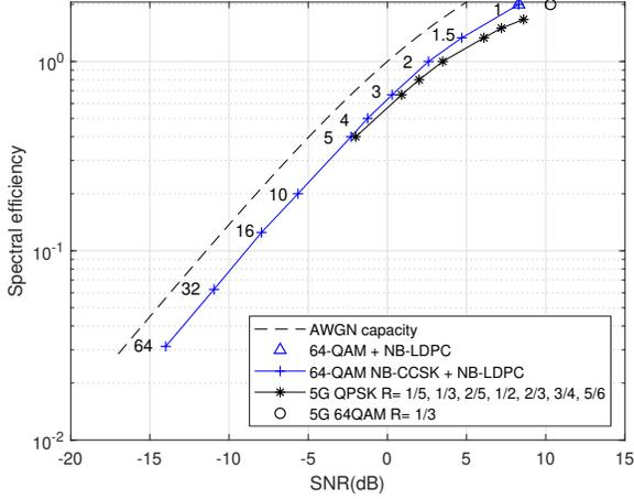
Fig. 8. Spectral efficiency of NB-CCSK(64) with 64-QAM modulation
