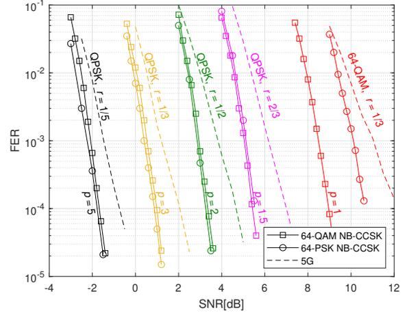
Fig. 7. FER of 64-QAM and 64-PSK TCCSK
