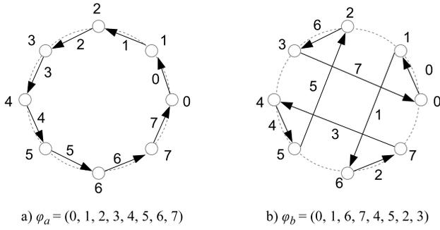
Fig. 3. Permutation of an 8-PSK NB-CCSK sequence
