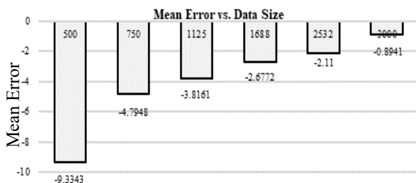
Fig. 5. Mean error variation vs. data size considered for training a feedforward neural network with one hidden layer and 11 neurons
