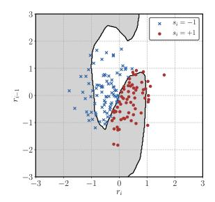
Fig. 4. Decision boundary of proposed CNN equalizer with nonlinear channel  $h = [1, 0.5], g(v) = v - 0.9v^3$  and SNR = 1.
