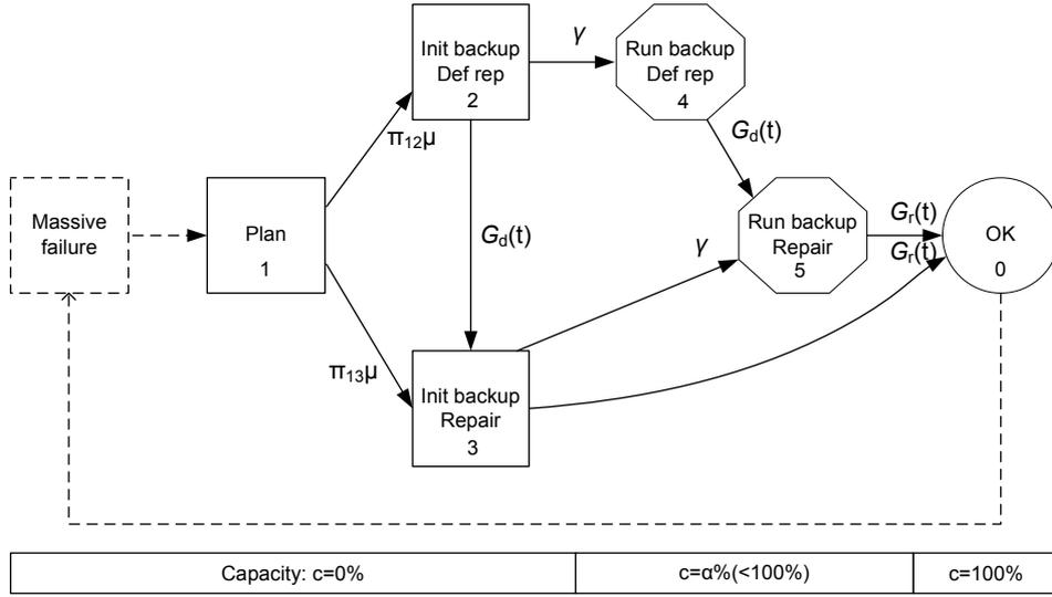
Fig. 1. Survivability model with 6 phases for the example.
