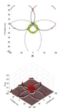
Figure 4. Source Localization Result for Source 1, a) A 2D radial basis location estimation for different nodes, b) A 3D probability space for source localization
