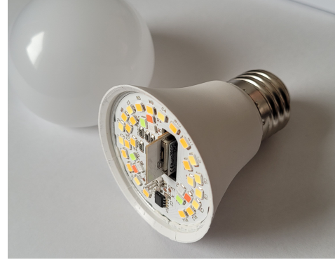
Figure 1. A photo of a typical consumer grade ‘Tuya’ compatible smart light bulb that we use for our NIDS light bulb demonstration 2
