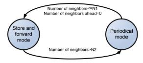
Fig. 4: Two mode model and switching mode conditions
