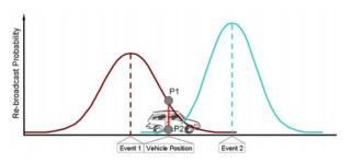
Fig.2: The vehicle receives two event notifications. The utility of event 1 is higher so the probability of rebroadcasting this event is higher
