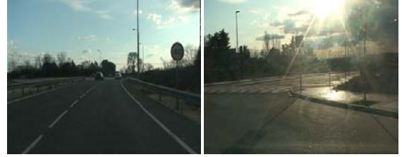
Fig. 10. Example of misdetections due to shadows (left) and dazzling (right).
