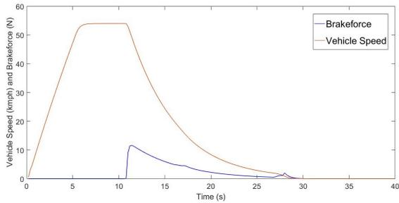
Fig. 8. Use Case 1: Profiles of vehicle speed and brake pedal force
