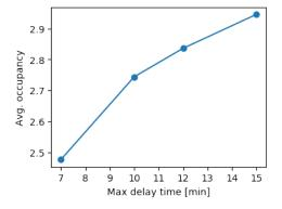
Fig. 6. Relation between maximum travel delay and the average vehicle occupancy.
