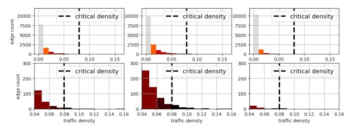
Fig. 4. Histogram of traffic densities in the three different scenarios. In the second row, only the bins with traffic density above 50% of critical density  $(0.04 \, \mathrm{vehicle} \, \mathrm{m}^{-1})$  are shown to improve readability. Edges with zero traffic density were discarded from all histograms.
