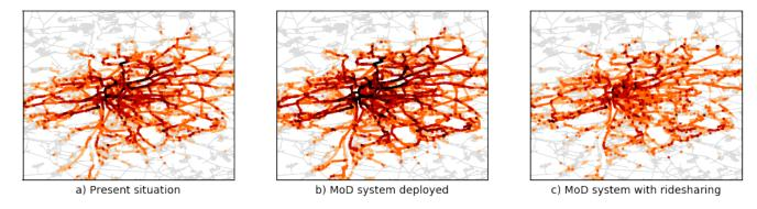
Fig. 3. Comparison of traffic densities over the road network in the three compared scenarios. The darker colors indicates higher traffic density, black color is reserved for the roads that are congested, i.e., the traffic density exceeds the critical density.
