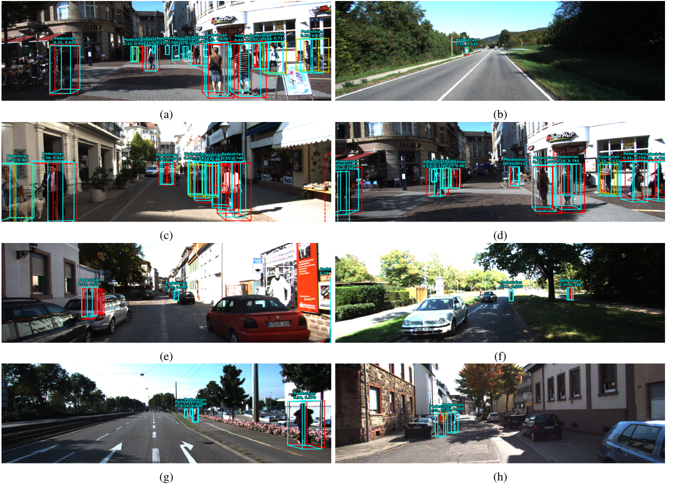
Fig. 3: Qualitative results for the proposed model on the KITTI validation set. The model can estimate the 3D location of people with different orientations and poses. (a) - (d): examples with good performance on crowded scenes, far away objects, occluded and truncated objects. (e) - (h): failure cases with missed detections, false positives and confusions with cyclists. Ground truth: red. Predictions: cyan. Numbers on top of boxes: detector objectness, IoU.
