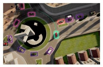
Fig. 5: Traffic scene showing the roundabout scenario. The green rectangle in the center is around the ego vehicle, and the dotted green line visualizes the currently chosen action for the agent. All other cars are surrounded by a rectangle colored according to their importance for the risk estimate, as assigned through integrated gradients, high importance is colored orange, unimportant dark purple or black.
