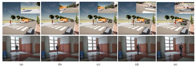
Fig. 5. Interaction example between pedestrian and virtual vehicle equipped with external HMI: (a) The pedestrian starts with their back to the crosswalk and is told to turn around when the vehicle approaches. (b) The pedestrian makes eye contact with the vehicle and hesitate to cross. (c) The external HMI switches from red to green. (d) The pedestrian enters the vehicle lane establishing the crossing event. (e) The pedestrian crosses the road.
