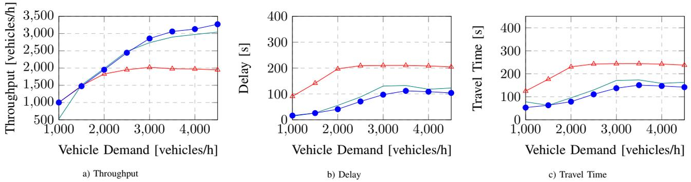
Fig. 6: Platooning Use Case (TL  $\blacktriangle$ , FCFS  $\text{—}$ , RB  $\bullet$ )
