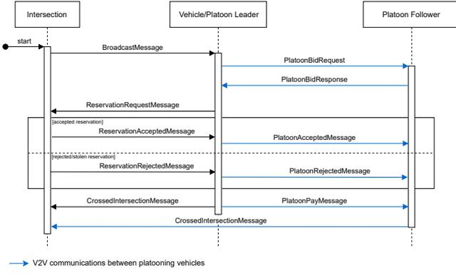
Fig. 2: V2X message flow of the intersection reservation mechanism
