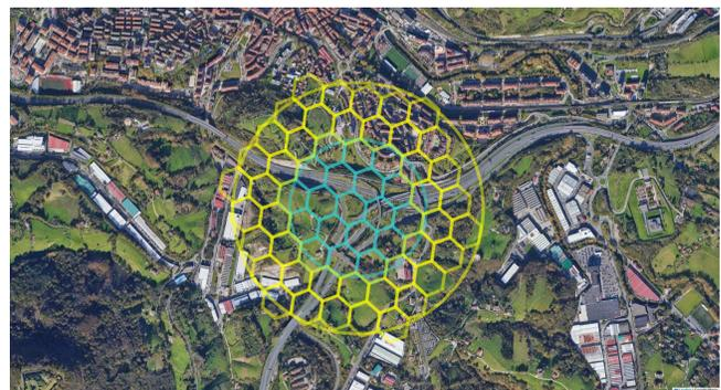
Fig. 2. H3 hexagon size for the selected resolution. Yellow hexagons represent indexes within the operating range, while blue hexagons represent those within the optimal range.
