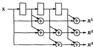
Figure 2: Architecture of the dual reciprocal duo-binary convolutional encoder
