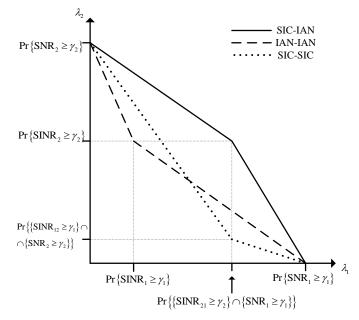
Fig. 4: Stability region comparison when condition (30) does not hold for both receivers.
