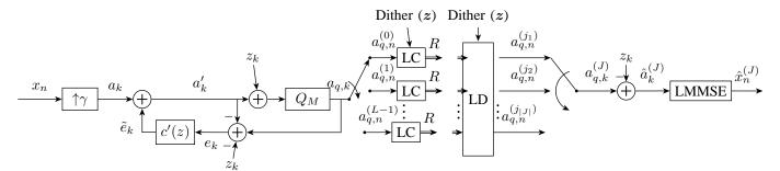
Fig. 1. The DSQ coding scheme. Illustrated on the left is the encoder, which produces L descriptions using oversampling and dithered quantization. Illustrated on the right is the decoder operation when a set  $J = \{j_1, j_2, ..., j_{|J|}\}$  of descriptions is received. LC and LD stand for lossless coding and lossless decoding respectively. The time index n corresponds to the original sampling rate, while k corresponds to the oversampled rate.
