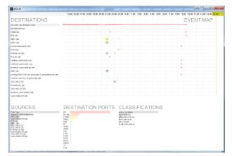
Figure 4. Port numbers encoded with colour, and overlaid onto events.
