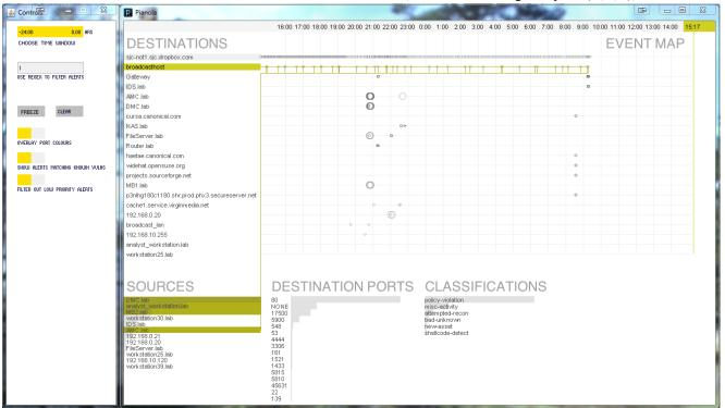
Figure 2. The main display of Pianola, highlighting events connected to one destination – 'broadcast host'. 'Event Map' is the main interface component, showing the timeline of multiple hosts on the network. Smaller sub-panels reveal information on Destinations, Sources, Ports and Classifications, and are linked to events in the Event Map through user actions such as selection and brushing. Finally, a control panel allows filtering operations and overlaying of colours on port data.
