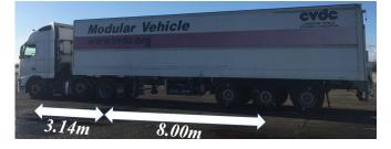
Fig. 1. Tractor-semitrailer test vehicle. Distances shown between the front axle and the hitch point for the tractor, and hitch to second rear axle for the semitrailer.
