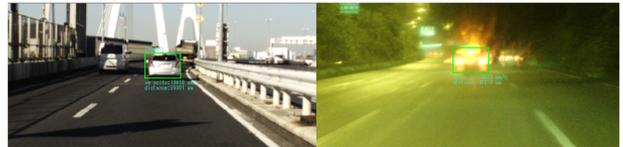
Fig.1 Detection results of our camera system. Left: Ideal environment for most research; Right: Bad environment in the real world. We focus on real world robustness at low cost using the camera-only system.
