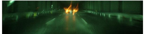
Fig.11 Image under test condition (30mm/h artificial rainfall)
