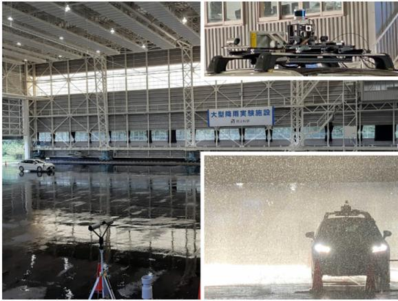
Fig. 4. The rainfall facility at NIED [32] where lidar point cloud and rainfall measurement data was collected from a stationary and moving vehicle in 15 mm/h and 50 mm/h rainfall rate setup. The rainfall area encompasses the entire hall which measures 65.4 m<sup>2</sup>. The disdrometer can be seen in the bottom-left of the figure. The sensor setup is shown in the top-right corner.
