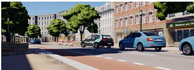
Fig. 4: View of the scenario simulation in OCTANE<sup>2</sup> showing a two-way street where one driving direction is blocked by a construction site. Vehicles in this direction have to drive on the opposite lane. In dense traffic, this requires an explicit stopping and yielding by the vehicles on the free lane.
