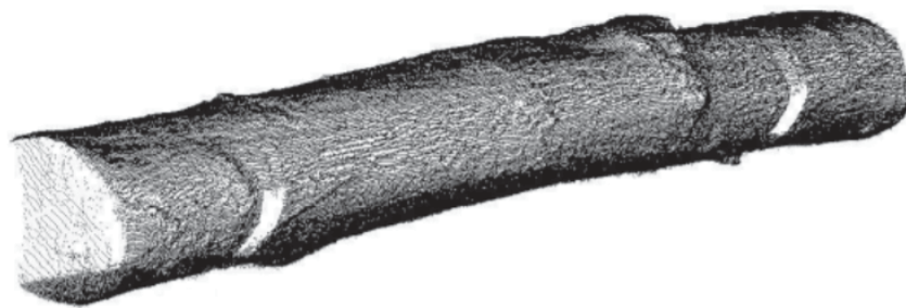
Figure 11. A sample point cloud image of a 3-D laser-scanned red oak log [23].
