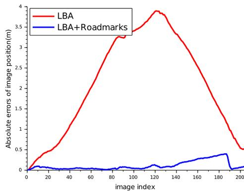
(c) Difference of localization methods with ground-truth.
