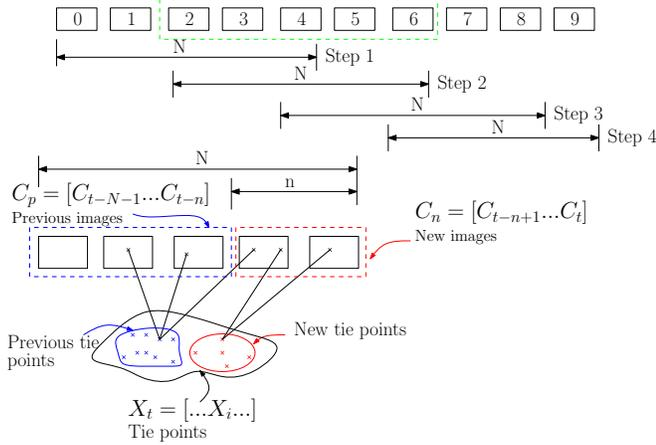
Fig. 5. Schematic flow of local bundle adjustment.
