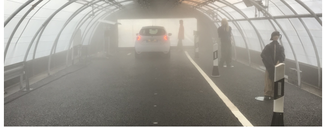
Fig. 1. Experimental setup in the climate chamber in fog with a visibility of 20-30m.
