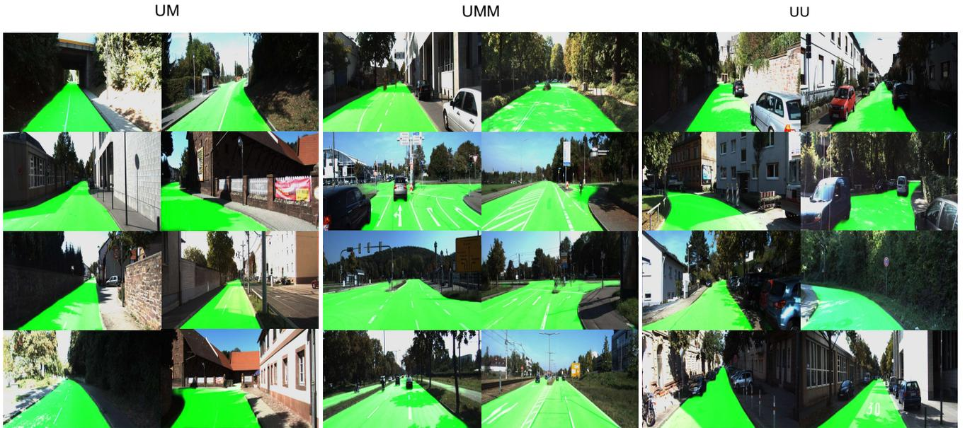
Fig. 5. Qualitative results of PLARD in different road scenes. Presented images show that PLARD is robust to severe illumination conditions. Best view in color.
