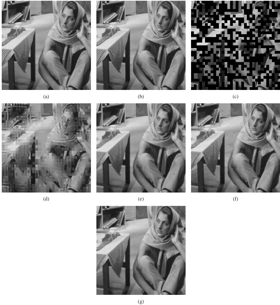
Fig. 3. (a) Original Barbara, (b) BDI inserted Barbara, (c) erroneous image received with 50% of block lost, (d) restored image from a spatial interpolation, PSNR=20.03 dB, (e) restored image from DCT coefficients, PSNR=29.89 dB, (f) restored image from the DWT coefficients, PSNR=31.05 dB, and (g) restored image from the hybrid scheme, PSNR=30.92 dB.
