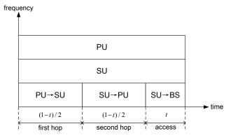
Fig. 2. Time slot allocation between a PU and a SU. PU and SU can transmit directly (on different subcarriers) or by a cooperation manner.
