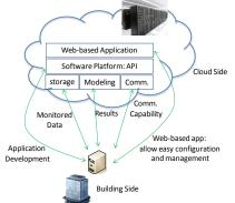
Fig. 14. Cloud computing components and interaction with the building side servers
