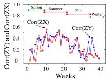
Fig.3. Correlations between electrical energy (Z), temperature (X), and humidity (Y)
