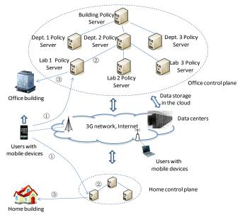
Fig. 13. Example dynamic multi-source energy-saving policy adjustment by the mobile devices
