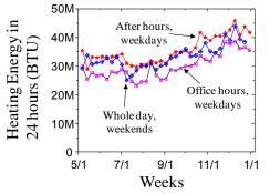
Fig. 8. Comparison of **heating** energy consumption averaged in 24 hours for office hours, after hours, and weekends
