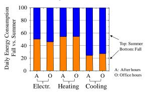
Fig. 11. The daily energy consumption comparison between Summer and Fall, considering after hours and office hours
