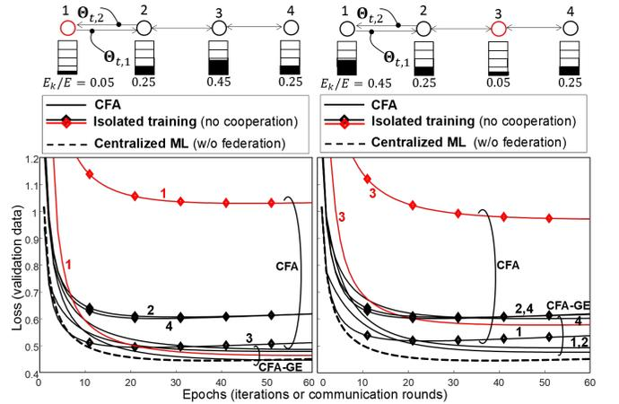
Fig. 4. Effect of non-IID unbalanced training data over device  $k = 1$  and  $k = 3$  (red lines) of a multihop wireless network composed of  $K = 4$  devices. Validation loss over the full MNIST dataset vs. epochs (or consensus iterations). Comparison between CFA (solid lines), isolated model training (diamond markers), and centralized ML without federation (dashed line) is also presented. Non-IID data distribution is shown visually on top, for each case.
