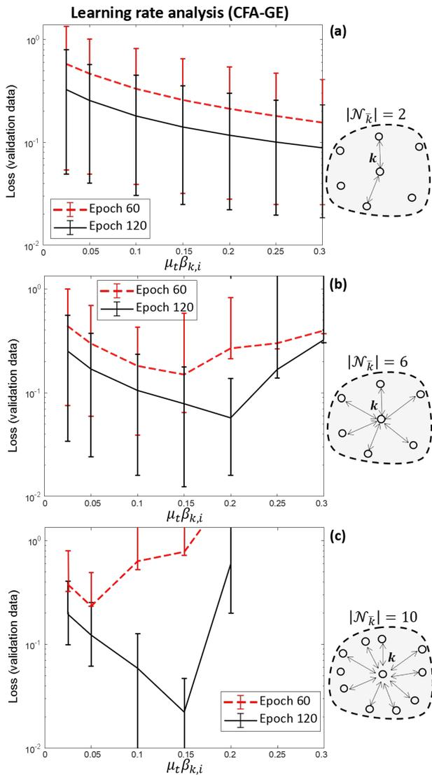
Fig. 7. From top to bottom: validation loss for varying rates ( $\mu_t \beta_{k,i}$ ) for  $K = 80$  devices and  $k$ -regular networks with varying connectivity, ranging from a)  $|\mathcal{N}_{\bar{k}}| = 2$ , b)  $|\mathcal{N}_{\bar{k}}| = 6$  up to c)  $|\mathcal{N}_{\bar{k}}| = 10$ .
