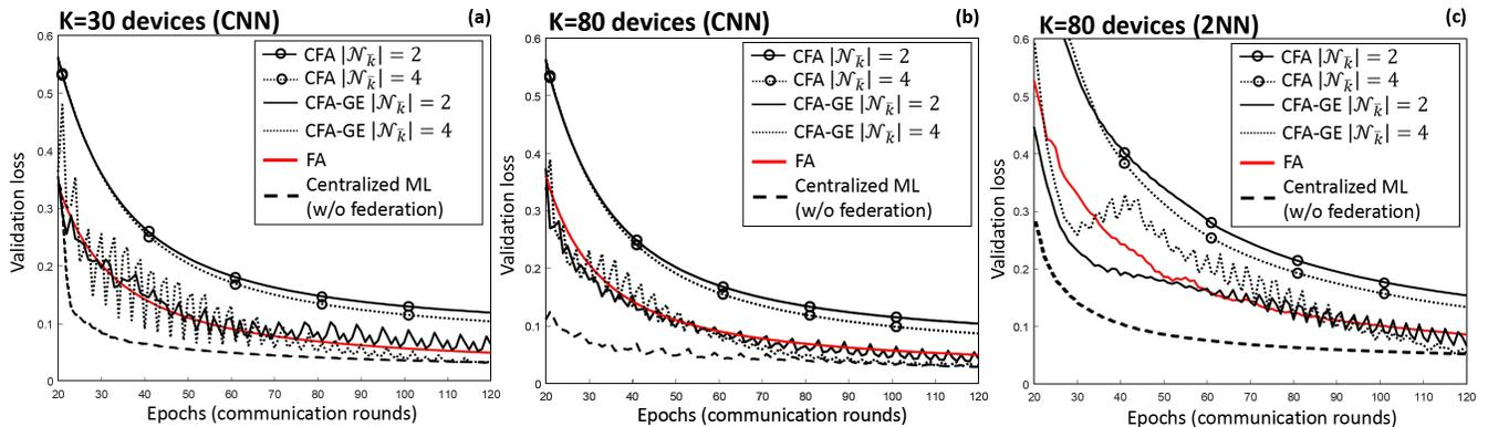
Fig. 6. From left to right: a) FL for CNN model with  $K = 30$ , b)  $K = 80$  devices and c) 2NN model with  $K = 80$  devices. The network is characterized by  $|\mathcal{N}_k| = 2$  (solid lines) and  $|\mathcal{N}_k| = 4$  (dotted lines) neighbors per node. Comparative analysis of CFA, CFA-GE, FA (red lines), and centralized ML *i.e.* learning w/o federation (dashed lines). CNN and 2NN parameters are described in Table I.
