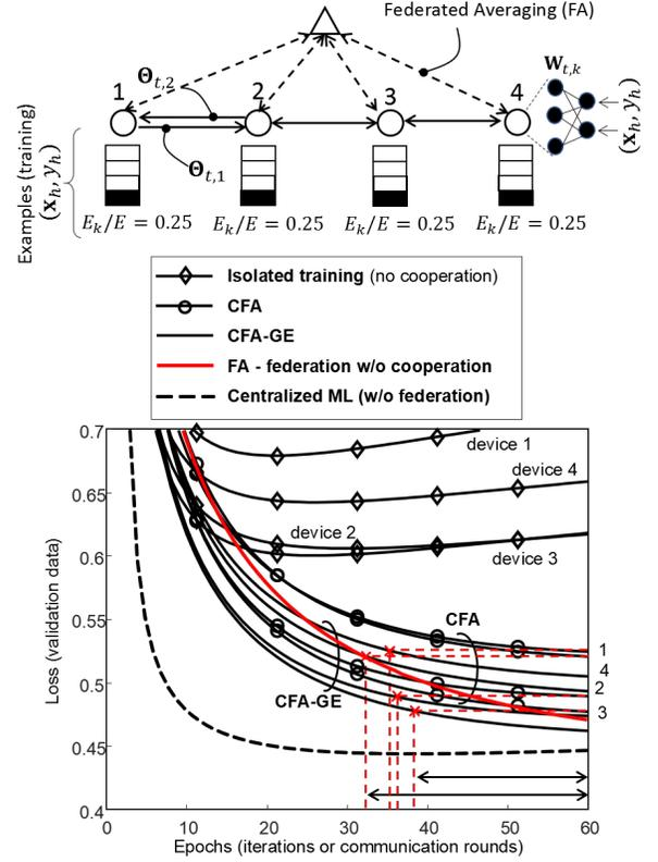
Fig. 3. Comparison of FL methods over a multihop wireless network of  $K = 4$  devices. Validation loss vs. iterations over the full MNIST dataset for all devices: CFA (circle markers), CFA-GE (solid lines without markers), FA (red line), isolated model training (diamond markers), and centralized ML without federation (dashed line). Iterations correspond to *epochs* when running inside the server, or *communication rounds* when running consensus or FA.
