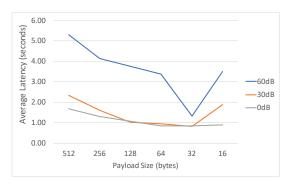
Fig. 14: NB-IoT Latency from Attenuated DRC to Smart Plug
