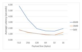
Fig. 13: NB-IoT Latency from DRC to Attenuated Smart Plug
