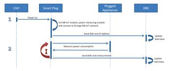
Fig. 4: Sequence Diagram to Report Measurement
