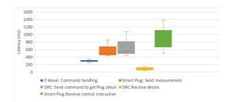
Fig. 10: Min-Max Latency Summary of Different Activities at 0 dB Attenuation
