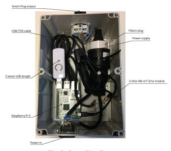
Fig. 3: Smart Plug Prototype
