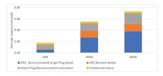
Fig. 9: Communication Latency of Setting Appliance's Status
