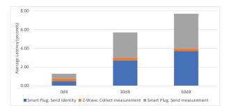
Fig. 8: Communication Latency of Reporting Measurement
