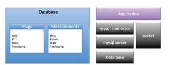
Fig. 7: DRS Software Architecture and Database Schema
