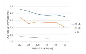
Fig. 11: NB-IoT Latency from Smart Plug or DRC to DRS
