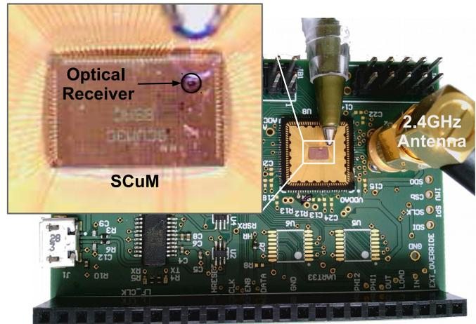
Fig. 1. Development environment of the Single Chip Micro Mote ( $SC_{\mu}M$ ), a  $2\times 3\times 0.3$  mm<sup>3</sup> crystal-free mote-on-chip, which features an ARM Cortex-M0, an IEEE802.15.4 radio operating at 2.4 GHz, and an optical receiver for programming [12]. Once the firmware is loaded onto the  $SC_{\mu}M$  chip, the chip can then be removed from its development board; all it needs to operate are a power source and an antenna.
