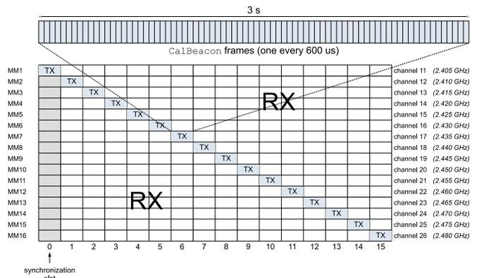
Fig. 12. The QuickCal Box schedule. Each OpenMote (numbered MM1–MM16) is assigned a different frequency channel. One after the other, each OpenMote sends 1,000 `CalBeacon` frames, one every 600  $\mu$ s. Slot 0 is used by MM2–MM16 to synchronize to MM1 by listening to its `CalBeacon` frames. Whenever an OpenMote does not transmit `CalBeacon` frames, it listens for `CalProbe` frames, to which it answers with a `CalAck` frame.
