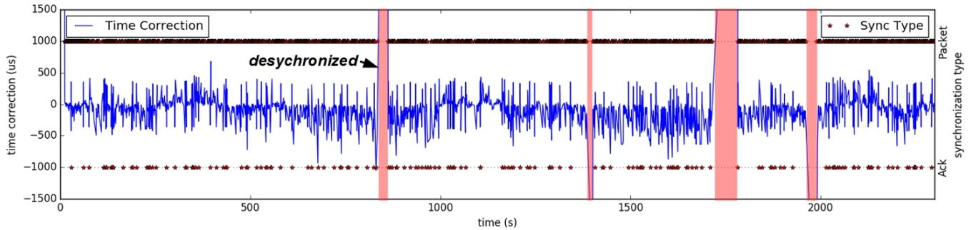
Fig. 17. Time correction of  $SC\mu M$  against an OpenMote while they form a heterogeneous 6TiSCH network. We use the OpenWSN implementation, which we have ported to the  $SC\mu M$  chip.  $SC\mu M$  de-synchronized 4 times during the experiment but re-synchronized quickly.
