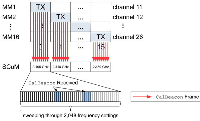
Fig. 13. QuickCal Step 1: receiving from the QuickCal Box. SC $\mu$ M sweeps its frequency settings while listening for CalBeacon frames sent on all 16 frequencies by the OpenMote devices in the QuickCal Box. OpenMote MM1 sends CalBeacon frames on channel 11 in slot 0, OpenMote MM2 sends CalBeacon frames on channel 12 in slot 1, etc. The SC $\mu$ M chip receives beacons at multiple frequency settings; it uses the algorithm in Section IV-C3 to determine the best setting.
