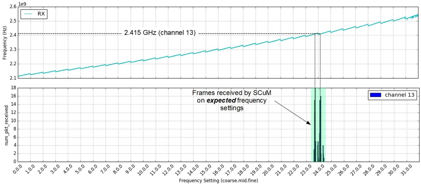
Fig. 8. Results of RX calibration (OpenMote  $\rightarrow$  SC $\mu$ M) on channel 13. The top plot shows the frequency SC $\mu$ M receives on. The bottom plot is a histogram of the number of frames received by SC $\mu$ M for each frequency setting.
