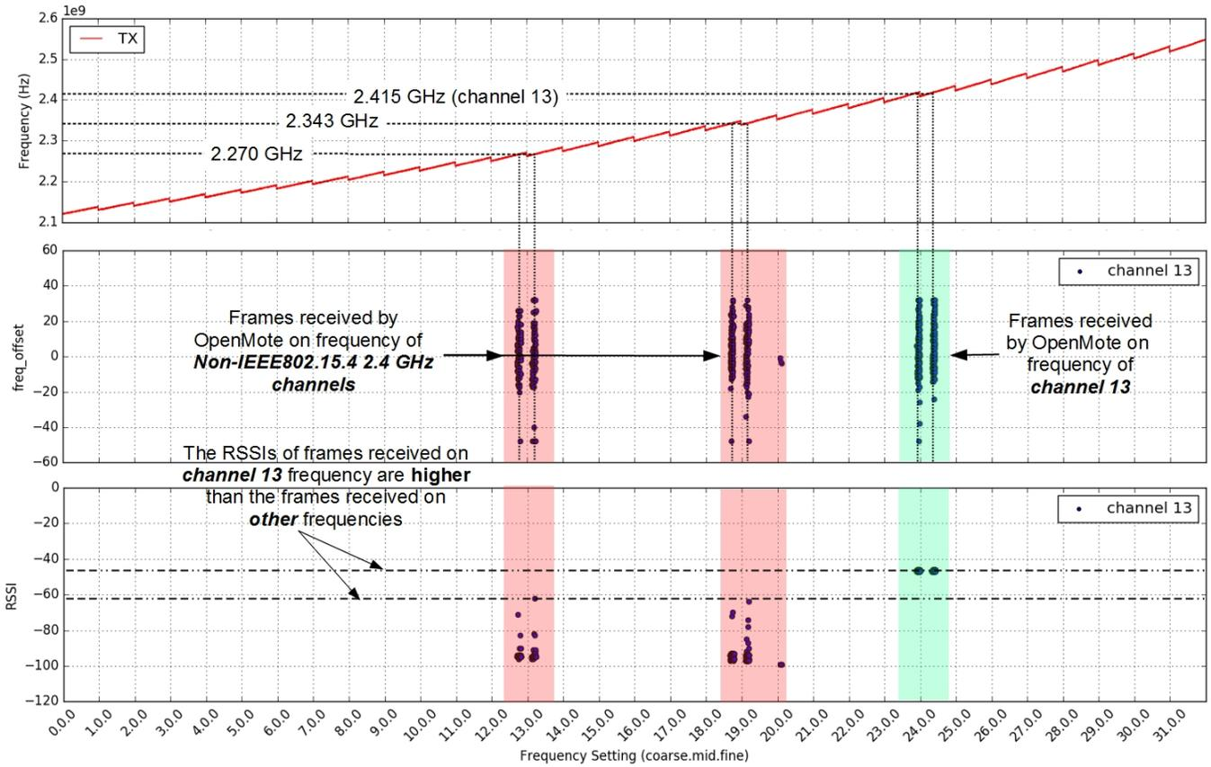
Fig. 7. Results of TX calibration (SC $\mu$ M  $\rightarrow$  OpenMote) on channel 13. The top plot shows the frequency SC $\mu$ M transmits on, as in Fig. 4. Each dot in the bottom plots indicates that the OpenMote has received a frame; these plots shows the frequency offset and the RSSI for that frame.
