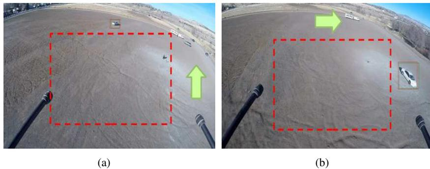
Fig. 6: The target (e.g., a white car) is detected outside of the detection region, the UAV would move forward (shown in (a)) or move right (shown in (b)), and try to make the target be inside the detection region.
