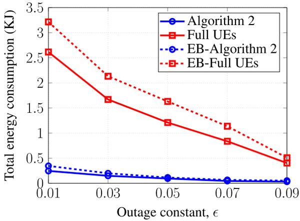
Fig. 8. Total energy consumption versus the outage constant.
