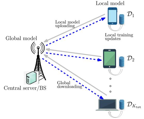
Fig. 1. Illustration of the FL-enabled wireless IoT network.
