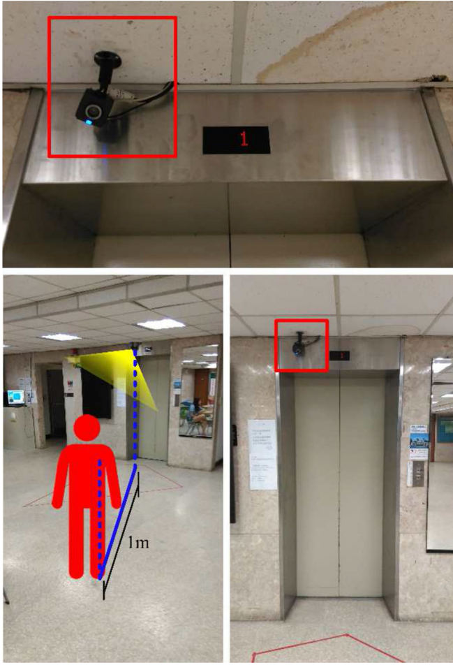
Fig. 7. Actual set-ups for the performance test of the thermal imaging sensor conducted at the buildings of Department of Geography in NTU.
