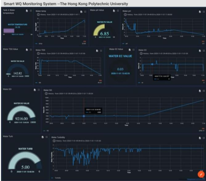
Fig. 5. The ThingsBoard web-server dashboard of the developed IoT system.
