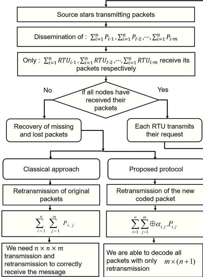
Fig. 3. Phases of operation of the proposed protocol.
