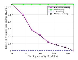
Fig. 10. The expected weighted-sum energy versus the caching capacity constraint with  $T=3.5\mathrm{s}.$
