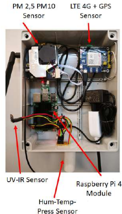
Fig. 7: Prototype of the environment monitoring sub-system.
