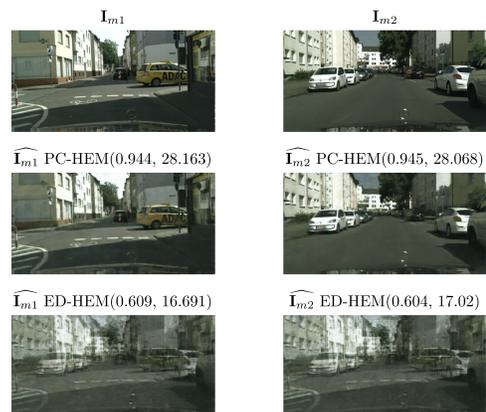
Fig. 10: Comparison of image recovery effect between PC-HEM and ED-HEM schemes, with parameters  $v1 = 0.4$ ,  $v2 = 0.1$ ,  $P = 35$  dBm,  $d_{SR} = d_{RD} = 50$  m. where, the numbers in parentheses indicate PSNR and MS-SSIM, respectively.
