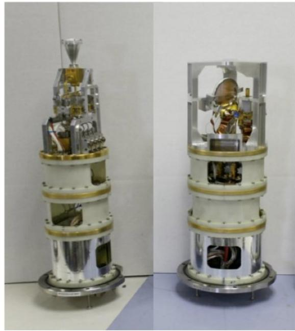
Fig. 6. Two of the cartridges for the ALMA Front End dewar. Left: Band 3 (84-116 GHz) cartridge. Right: Band 7 (275-373 GHz) cartridge.
