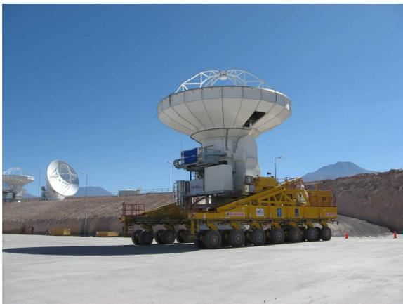
Fig. 3. The first antenna accepted by ALMA from Vertex is moved to a pad near the Operations Support Facility Technical Building on one of the transporters. In the background are the first antenna accepted by ALMA, from Melco, undergoing holography tests on the right, and Vertex No 4 on the left.
