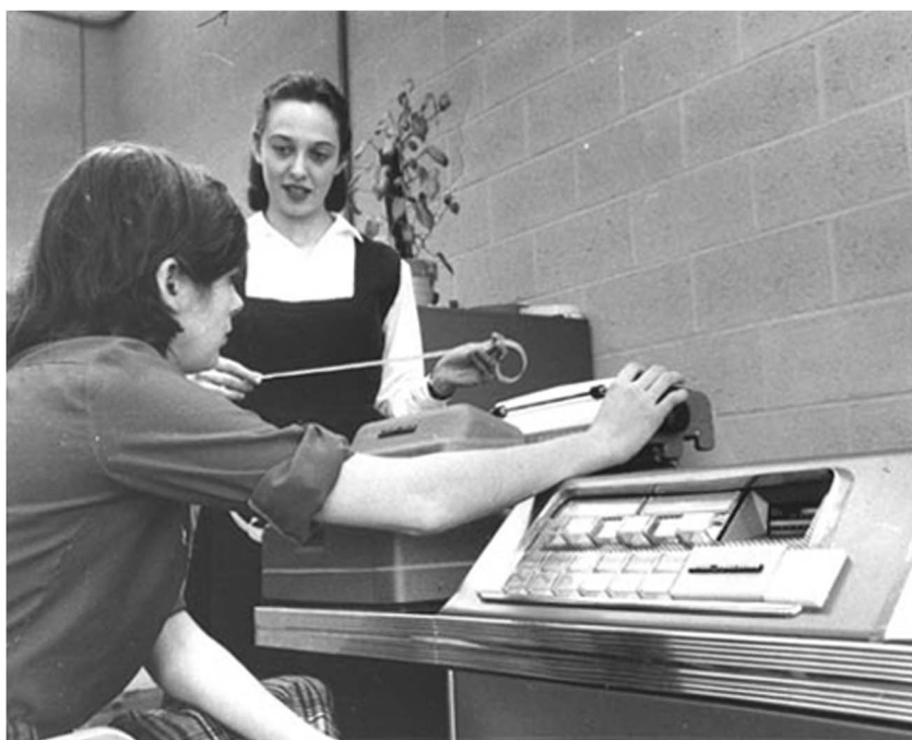
Fig. 1. A teacher holds a segment of paper tape while a student sits at the Flexowriter with his right hand on the carriage. The Librascope LGP-30 control buttons are on his right. Courtesy of the Computer History Museum.
