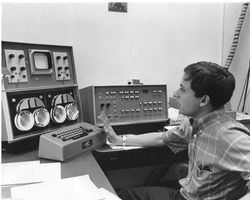
Fig. 3. Maury L. Pepper of the Washington University's Computer Systems Lab in St. Louis, MO, USA, developed a floating-point arithmetic subroutine on its LINC in the mid-1960s. Courtesy Maury L. Pepper.
