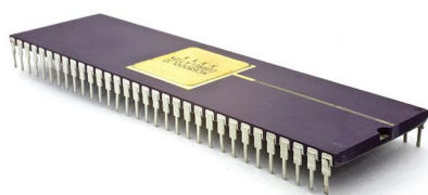
Fig. 7. Motorola's 68000 series microprocessor is less than 2.5 in or 62 mm long, but the 16/32-bit hybrid architecture of the computer chip under the square heat spreader makes it the equal of classic minicomputers. It is still in production in 2012. Copyright Mark Richards. Courtesy of the Computer History Museum.
