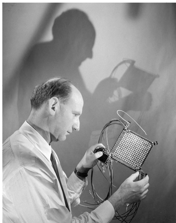
Fig. 4. Jan Rajchman holds RCA’s first ferrite core memory panel, a 16 \times 16 matrix using magnetic ribbons wrapped around spindles. This memory is on permanent exhibit at The College of New Jersey’s Sarnoff Collection in Ewing, NJ, USA. (Courtesy David Sarnoff Library.)
