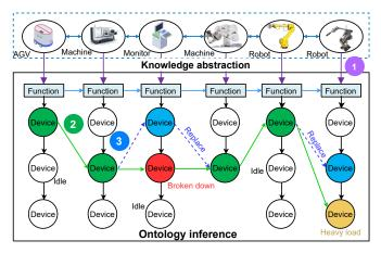
Fig. 8. Dynamic reconfiguration of manufacturing resources: 1) device selection by ontology reasoning based on the device function; 2) CM production line is constructed; 3) automatic switching to other devices from heavy-load devices or broken devices.
