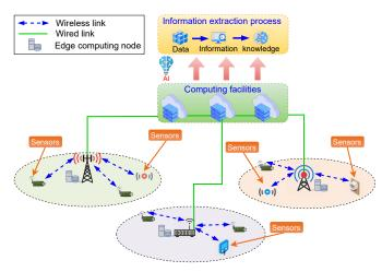
Fig. 5. Intelligent sensing based on edge AI computing. Sensor nodes collect ambient data while edge computing notes can preprocess and cache the collected data, which can be further transferred to remote cloud servers for in-depth data analysis.
