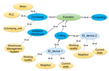
Fig. 4. Manufacturing resources from the device function perspective. The CM resources of a product can be mapped into computing, cutting, conveying, and other functions.
