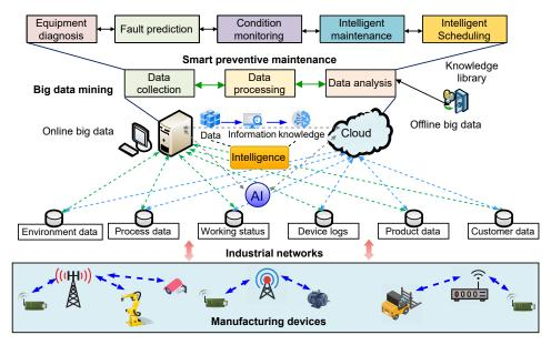
Fig. 11. Big data analysis using AI technology for smart preventive maintenance. The smart preventive maintenance system consists of CM devices, industrial networks, big data processing center, and applications for preventive maintenance. The data pipeline consisted of three main steps, data collection, data processing, and data mining and analysis using AI.
