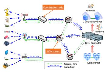
Fig. 6. Software-defined industrial networks consist of network coordinated nodes, SDN routers, SDN controllers, data centers, and cloud computing servers which can support intensive computing tasks of AI algorithms.
