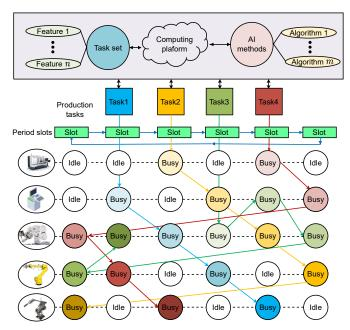
Fig. 9. Self-organization of schedules of multiple production tasks consists of three steps: task analysis, task decomposition and task execution.
