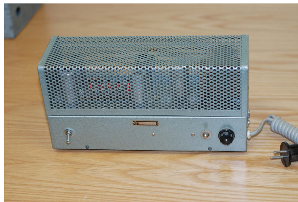
Fig. 3. “Ape,” aperiodic radio receiver used to identify and capture illegal agent radio traffic. Photograph by Johan Antus.
